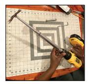
**12.** Attached the completed Assistant Tool 1 flap sander assembly to your chosen power tool and start!
