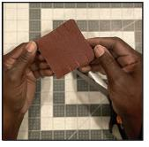
**3.** On 2 opposite sides of each square, cut a series of 1/2" slits 5/8" (16mm) apart. These "fingers" create flexibility and adhere closely to the surface as you sand.
