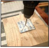
**4.** Using a hole punch or drill, make a 3/16" (5mm) hole (NO BIGGER) in the 4 squares.
