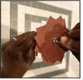
**11.** Ensure the sandpaper is fanned out equally before tightening with a Phillips head screwdriver.
