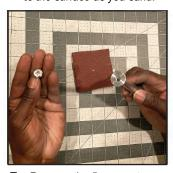
7. Remove the 5mm center screw located at the top of Assistant Tool 1.
