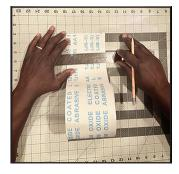
Cut sheet strips or a roll of sandpaper 3" (75mm) wide by 2" (50mm).
