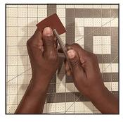
**3.** Place the creased sandpaper fold into the bottom of the slot of the Assistant Tool 2 at the narrow 1/4" (3mm) end.
