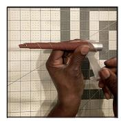
4. Using 1/2" tape, securely tape the end of the sandpaper to the tool to prevent slippage or loosening.
